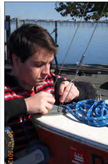
Bryan replacing the frayed wire that secures the jib tack. Photo by Chris Von Guggenberg.
