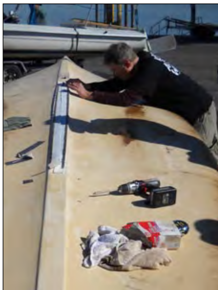
Dedicated members labor over Suzie Q's new centerboard gasket. Photos by Chris Von Guggenberg.
