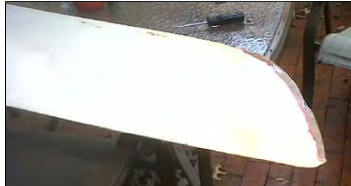
The damaged centerboard. Photos by Julian Mallott.
