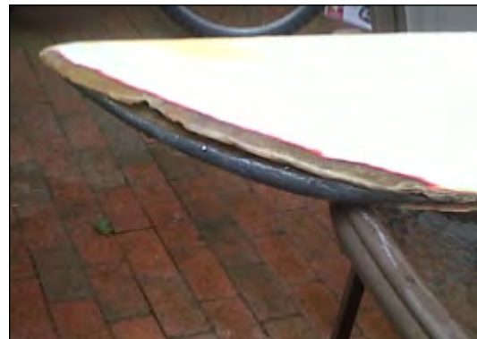
The damage to the centerboard is so significant that the lead ballast is exposed.
