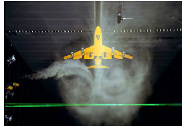
A test at Langley Research Facility shows the trailing vortices on a Boeing 747 model, using stationary smoke.
