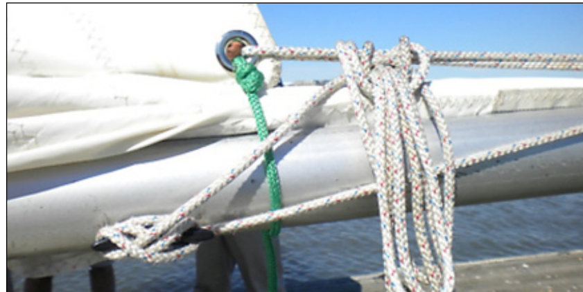
Securing the outhaul with the cleat found on the boom of all our Scots except Elisse.
