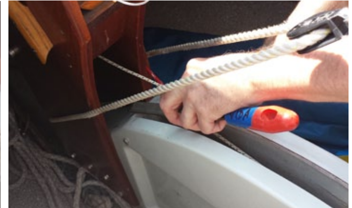
On Maintenance Day, all of the Flying Scot steel centerboard cables were replaced with fiber line, because over time the steel cables had become frayed, leaving strands of steel exposed which could slice into the exposed fingers of unsuspecting crew.
