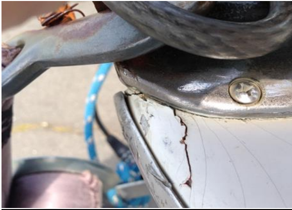
Photo showing damage due to hard docking on the nose.
