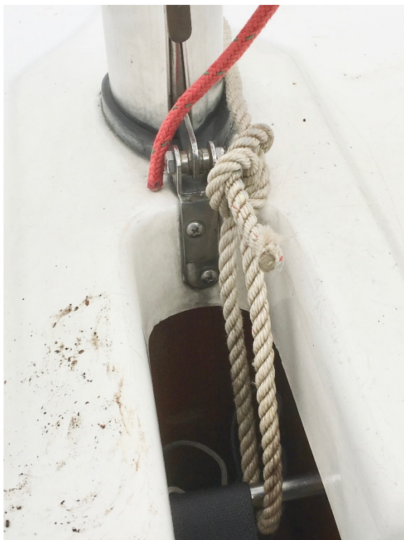
Figure 1. Anchor line coming from the bow eye is tied around the bridle bolt using a bowline.
