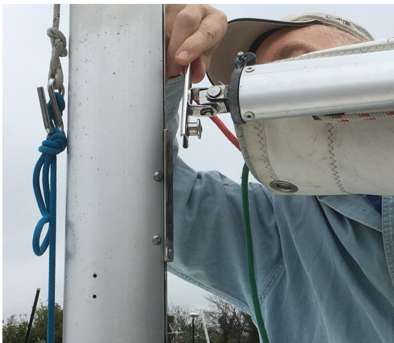
Figure 2. Fitting on the gooseneck that allows you to remove the boom. Pull out on the button below the gooseneck and slide the gooseneck up.
