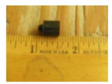
The image at left is a blown up picture of a **braking tip**. It's a small, black hard rubber cylinder which fits into holes on the side of the winch halyard housing and is held in place by the **backlash spring**.
