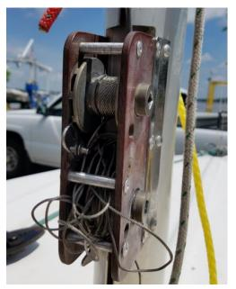
For those who are unfamiliar with the term "bird's nest", the image at left is a great example of the tangled mess that can occur if the halyards are not deployed properly or when the **brake tips** are worn out or missing.
