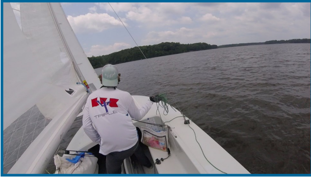
Sheet is routed outside the shroud and neatly coiled for throwing. As I initiate the tack, Ethan simultaneously releases the port jib sheet with his left hand as he starts his throwing motion with his right hand.
