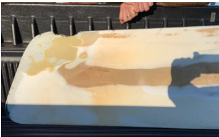
EXAMPLE OF DAMAGE TO A CENTERBOARD. THE DIFFERENT COLORS REPRESENT MULTIPLE REPAIRS.
