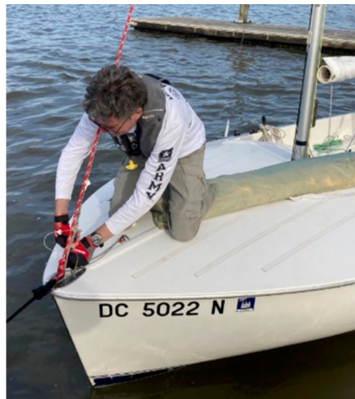
ALLEN RIGS A SECOND JURY RIG LINE BETWEEN THE BOW EYE AND THE LOWER END OF THE FORESTAY TO FURTHER SECURE THE FRONT OF THE MAST. PHOTO CREDIT: ERIC SCHMIDT
