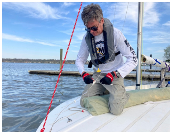
ANDIAMO BACK SAFELY. THE RED LINE CONNECTS THE JIB HALYARD TO THE BOW EYE TO SERVE AS AN IMPROVED FORESTAY. PHOTO CREDIT: ERIC SCHMIDT
