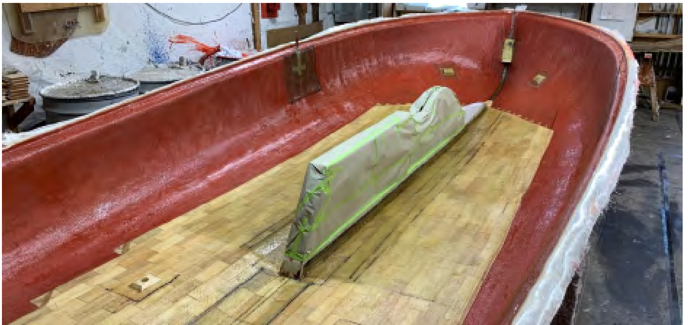
Hull in the mold – balsa laid out – ready for next layer of fiberglass
