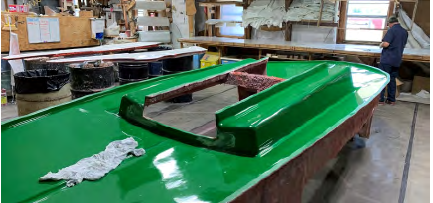
FS deck upside down being prepared to seal with hull
