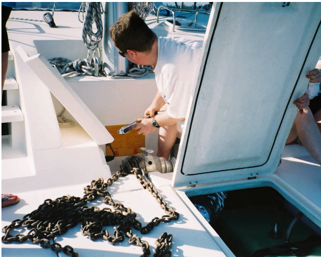
A windlass in operation bringing in the anchoring chain
